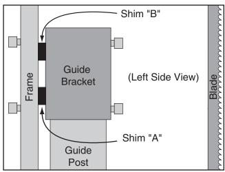
Figure 69. Location for placing shims.
